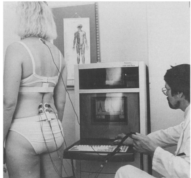
Fig 2. The set-up of real-time monitoring of body sagittal flexion and extension, ie, lumbar-pelvic rhythm, with the help of surface EMG from the paraspinal muscles and electronic movement sensors fixed at the sacrum and at the thoraco-lumbar area.
